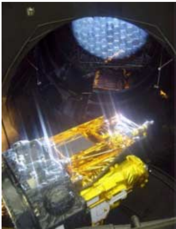
The INTEGRAL spacecraft inside ESTEC's Large Space Simulator during the thermal vacuum test (Summer 2002).
